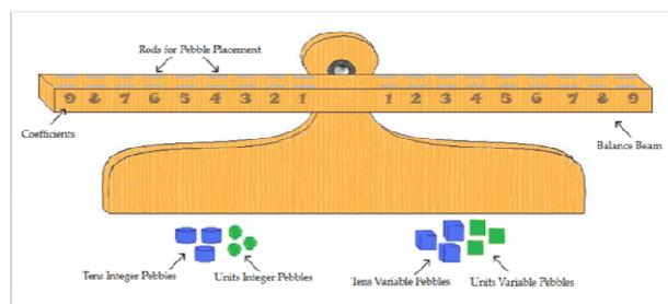
**figure 1.** The BEAM. The BEAM is constructed from one large wooden beam on a hinge. Rods are lined along the length of the BEAM for pebble placement. Each position is labeled with a number that represents that position's coefficient value. Pebbles come in two types denoted by shape (integers – round; or variables – square), and two amounts denoted by color (units – green; or tens – blue).
